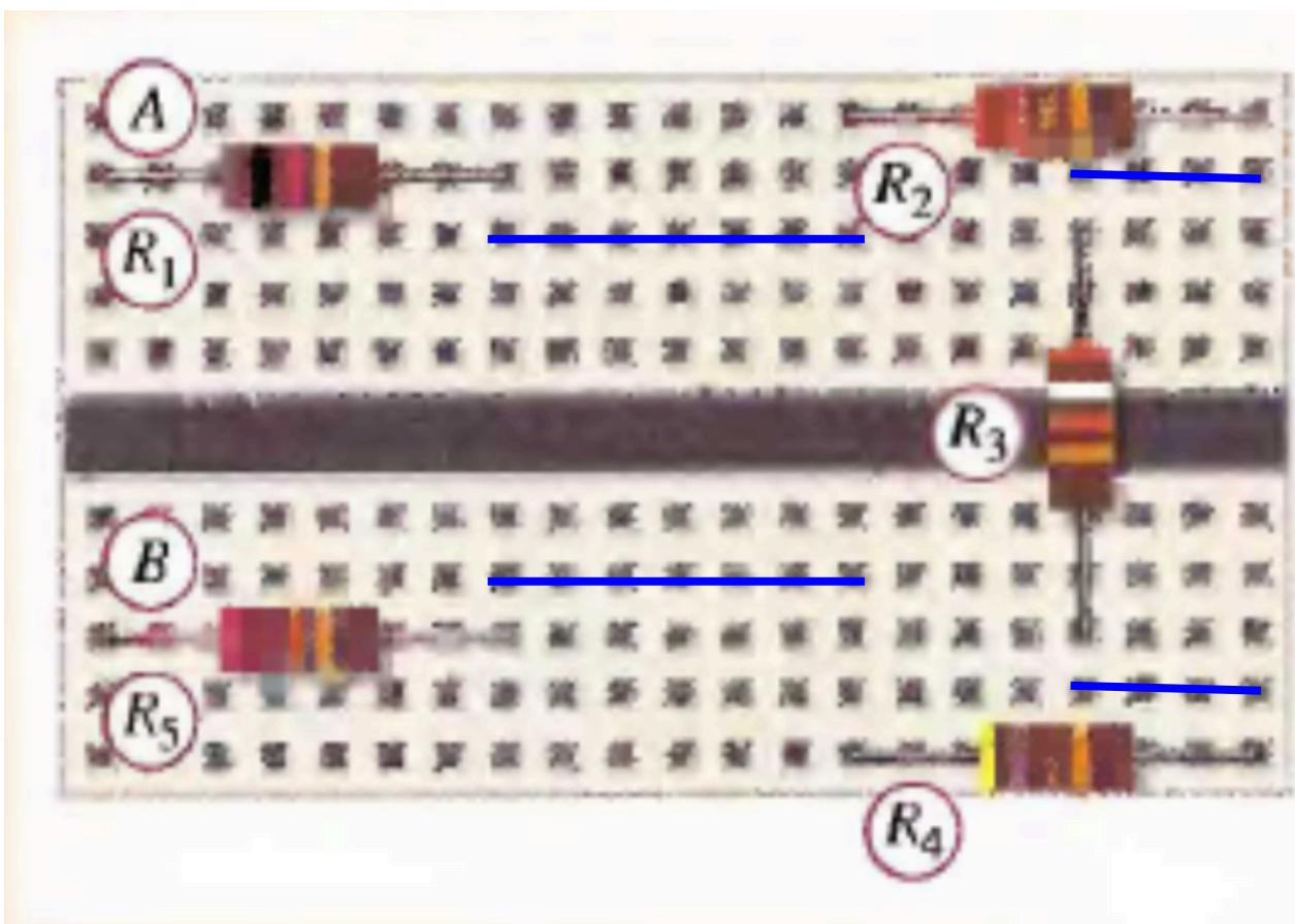
use jumper wire to connect & make it series circuit
