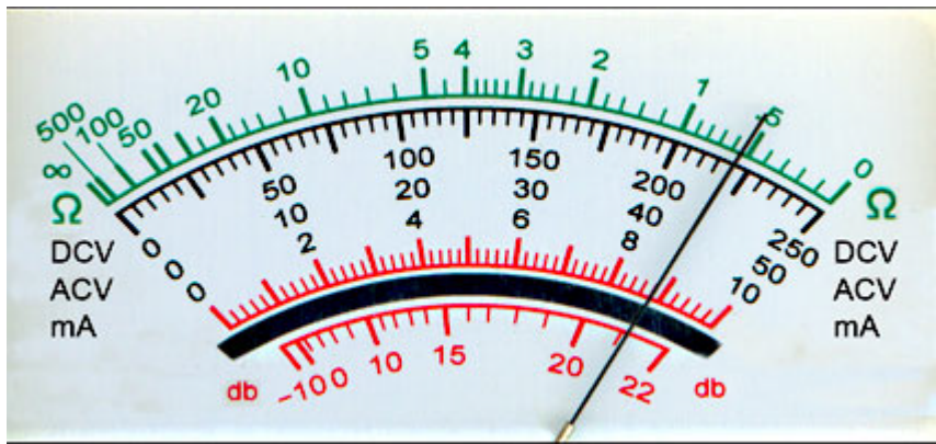
Figure 1.2 : Scale Meter for Analog Multimeter
