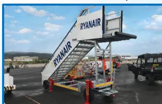
The mobile stairs at airports use hydraulics to move up and down.
