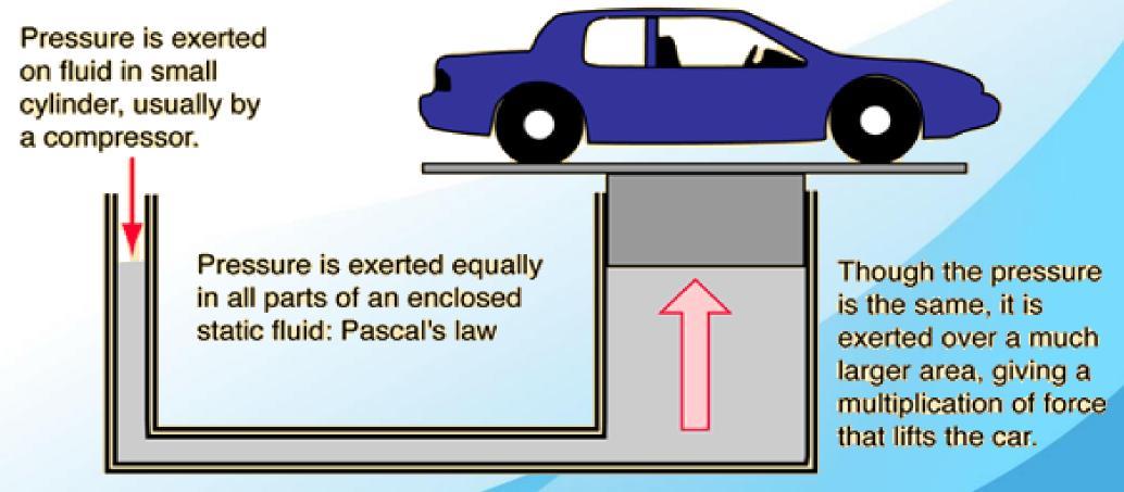
The force in the small cylinder must be exerted over a much larger distance. A small force exerted over a large distance is traded for a large force over a small distance.
